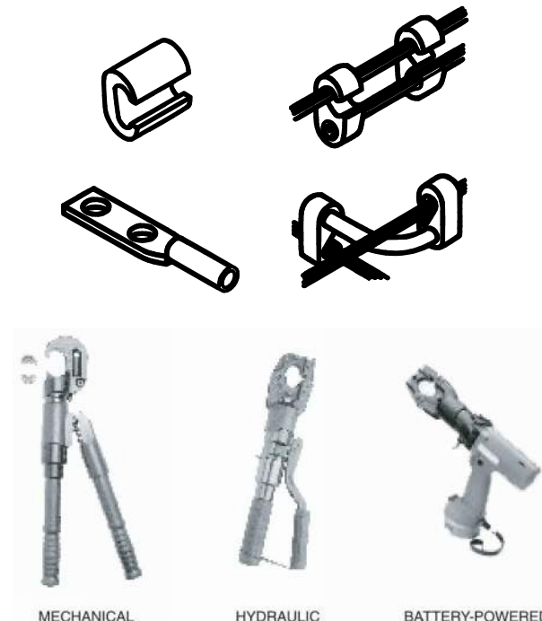
12 HIGH-COMPRESSION CONNECTORS AND TYPICAL CRIMPING TOOLS NOT TO SCALE
